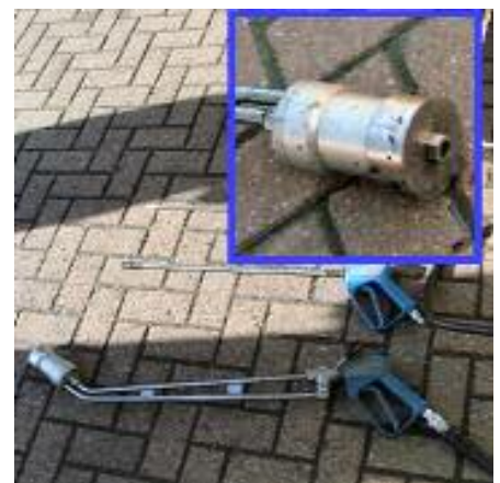
A selection of branches is available (the inset shows the fogging unit on the main branch)
