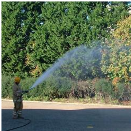
The unit can project liquid 25—30 metres.
